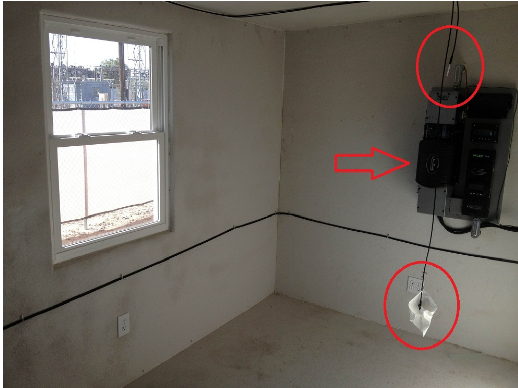
Figure 2.2.5: Indoor Air Temperature probes suspended roughly one foot from the floor and ceiling in the northwest corner of the structure. Paper shrouds are to shield the probes from window-source direct solar radiation in the late afternoon. A duplicate installation exists in the northeast corner of the structure.
