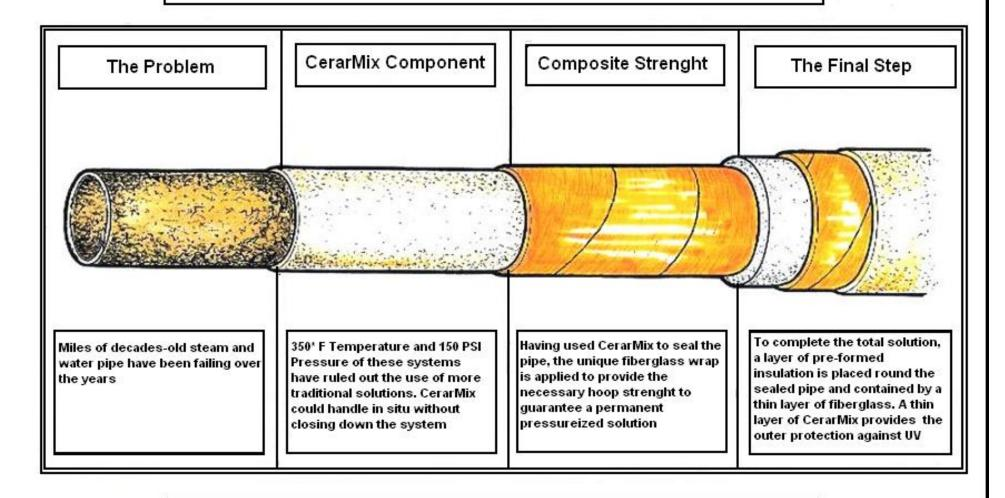
AMT Solution to the pipe effectively created a DURABLE SECOND PIPE enclosing the inner one, thus preserving the system integrity even after disintegration of the original pipe
