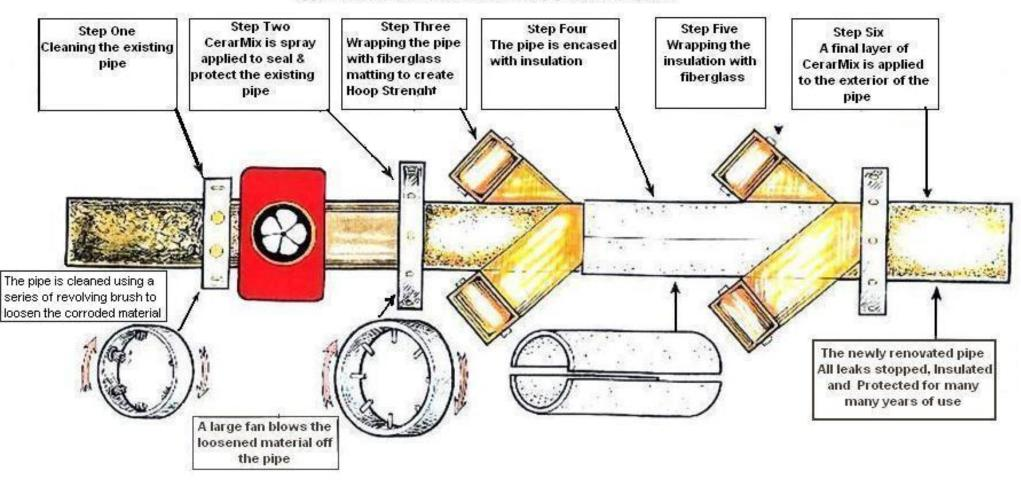
This ceramic composite solution allows for the combination of the positive tensile strenght qualities of fiberglass with the compressive strenght, water-proof and UV resistant characteristics of the CerarMix, creating a new strong, durable pipe using the existing pipe as a mold
