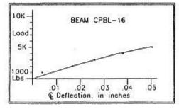
Close inspection of the plane of failure, involving measurement of the thickness of the AmTex at about 12 points, showed a mean coating depth of .096", leading to a stress on failure of the tensile coat of 4550 psi. This means that a working design allowable tensile stress of about 2500 psi is totally acceptable.
