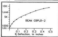
AmTex and fibreglass bottom and sides. Shortly before failure, the AmTex layer in compression peaked up at a node close to the loading plane. The failure, when it came, was also dramatic and sudden, at an ultimate load of 9680 lbs. Ultimate load in the AmTex/Fibreglass Composite would be about 12,000 psi in tension, so leading to 6750 psi for safe design.
