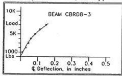
The first failure appeared to be slippage between the plain bar and the block, in one "short" end of the beam outboard of a loading plane, at about 5500 lbs. The tension layer of AmTex failed at 7300 lbs and then the gap progressively widening as the end hook at the short end rotated from the vertical.
